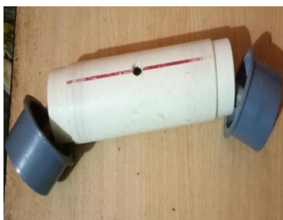
Fig. 2. Ohmic heating chamber for paddy
