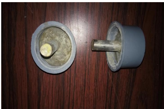
Fig. 4. Electrode using in ohmic heating model for parboiling of paddy
