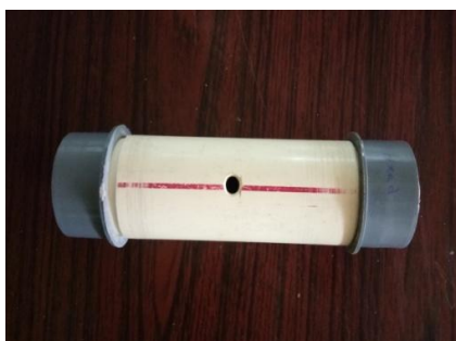
Fig. 2. Ohmic heating chamber for paddy
