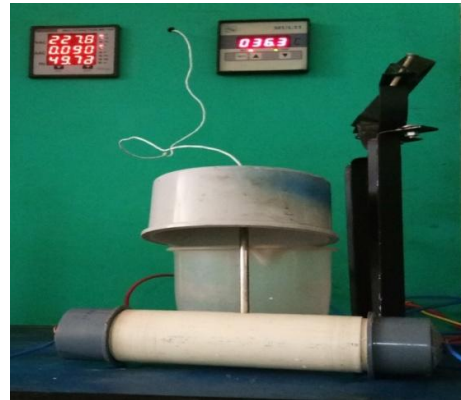
Fig. 6. Ohmic heating setup for parboiling of paddy
