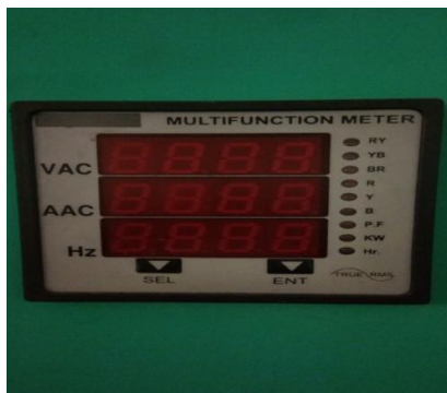
Fig. 5. Multi-function meter for ohmic heating system
