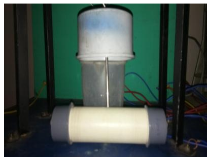
Fig. 3. Temperature controller and sensor for ohmic heating system
