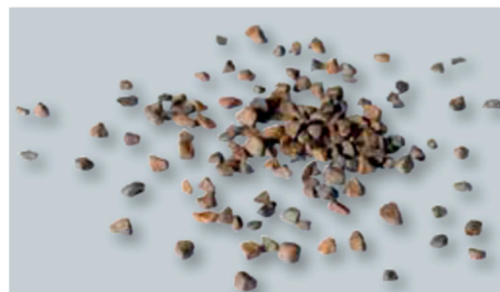
Figure 6. Medium in sizes 1.7–2.4 mm marked as KXMA 16 [17].
