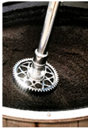
Figure 5. Spur gear as the workpiece mounted on Stream Finishing machine spindle [17].
