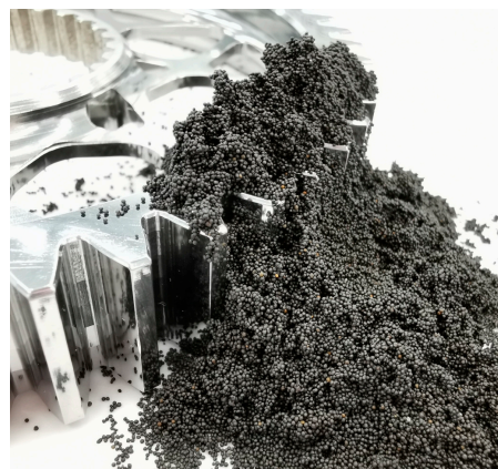
Figure 7. Medium size versus gear teeth module [17].
