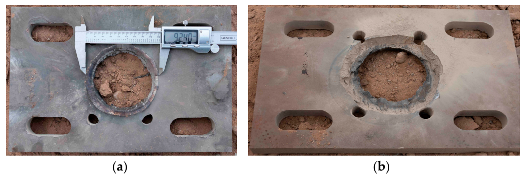
Figure 15. Shape of the witness plate after the test. (a) Front of the witness plate and (b) back of the witness plate.
