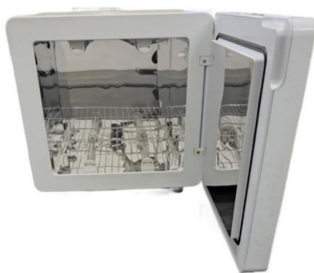
Fig. 3. UV-C light chamber with reflectors
