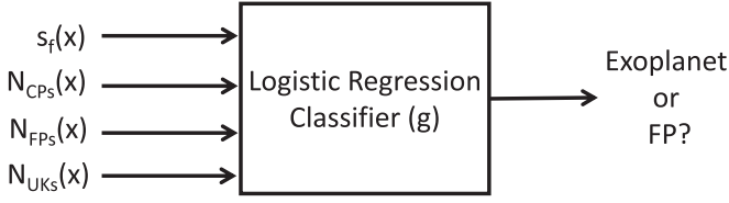
Figure 2. The machine learning model to boost the performance of a given classifier using multiplicity information.
