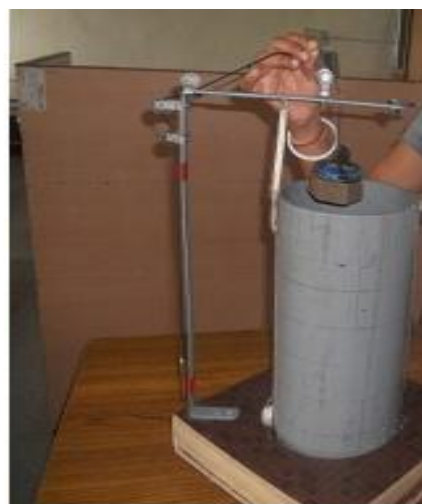
Plate 9. Placing the load on the SS plate
