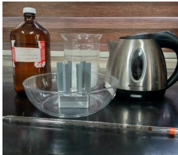
Figure 5. Improvised apparatuses/materials used for Acetone Vapor Smoothing. (adapted from [16]).
