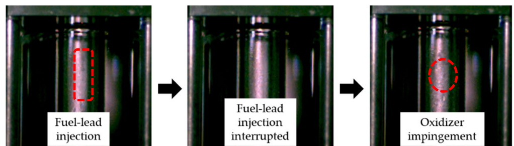
Figure 17. Interrupted fuel-lead injection in hard start.
