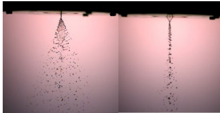
Figure 9. Shadowgraph images of injection spray by water (left: 0° angle, right: 90° angle).
