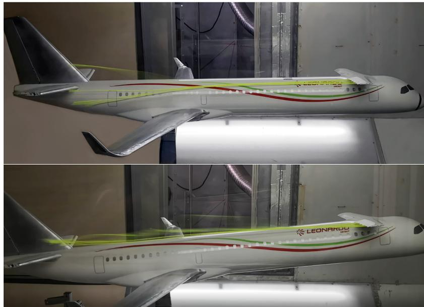
**Figure 14.** Canard wake impingement on the horizontal tailplane: visualization test through wool yarns.  $V = 35$  m/s,  $Re = 315,000$  at  $\alpha = 4^\circ$  and  $8^\circ$ .
