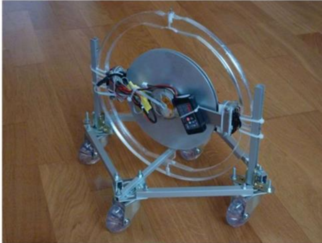
Fig. 5. Terrestrial Prototype II with rotating wheels, which allowed its direction control, with results similar to those of the submarine. 5
