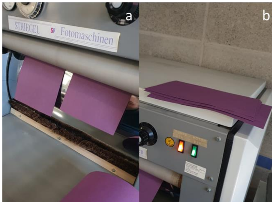
Fig. 6. Cover paper a) in the photo dryer, b) Cover paper after photo dryer
