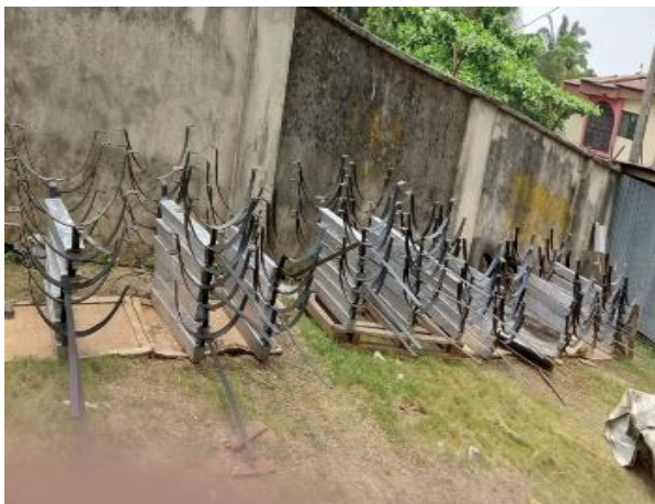
Fig. 2. Images of the fabrication of the anode-clamp assembly
