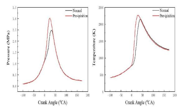
Fig. 1. Changes in cylinder temperature and pressure for normal combustion and pre-ignition [23]
