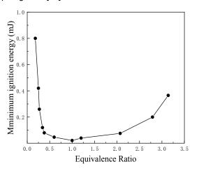
Fig. 2. The relationship between the equivalence ratio and the minimum ignition energy [34]
