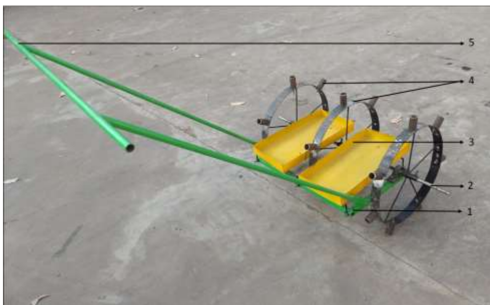
Fig. 1. Developed manually operated pull type three row dibble wheels
