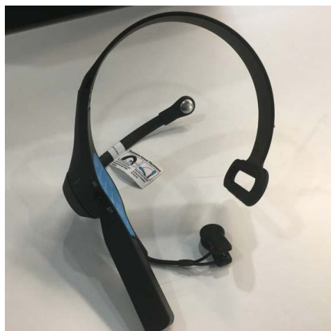
Figure 1. The NeuroSky Mindwave Mobile 2 EEG unit utilized for this project.
