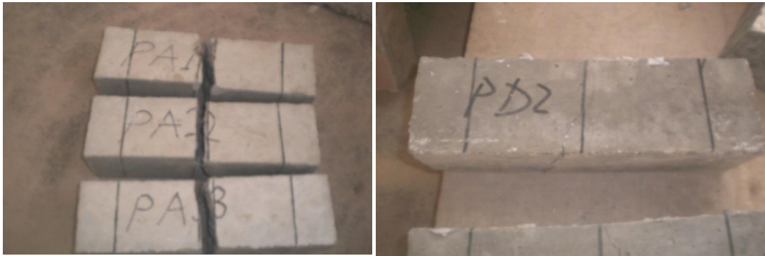
Fig. 8. Plain concrete prisms after failure Fig. 9. Polyethylene fibre concrete after failure
