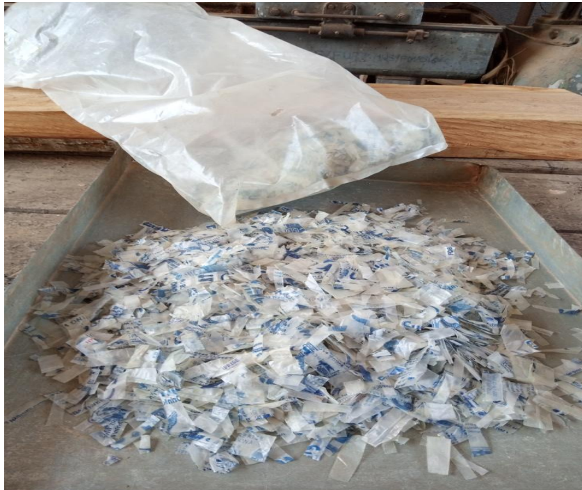
Fig. 1. Low density polyethylene fibres
