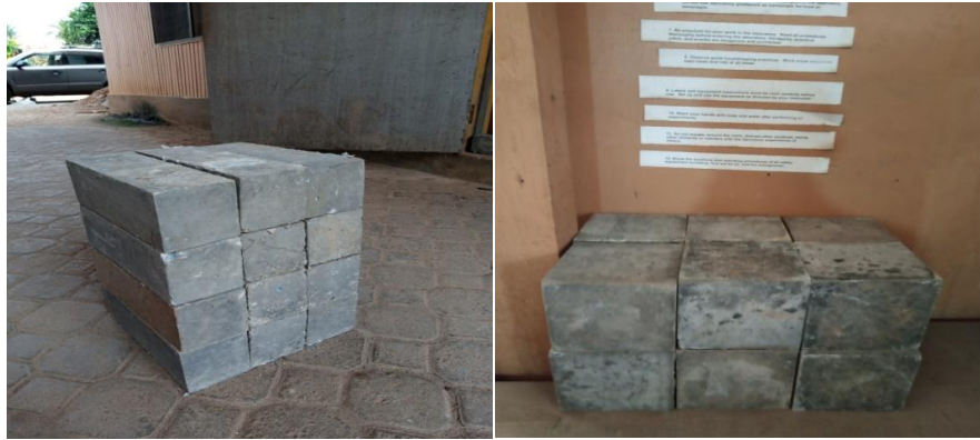
Fig. 3a. 100 mm × 100 mm × 300 mm prisms Fig. 3b. 150 mm × 150 mm × 150 mm cubes
