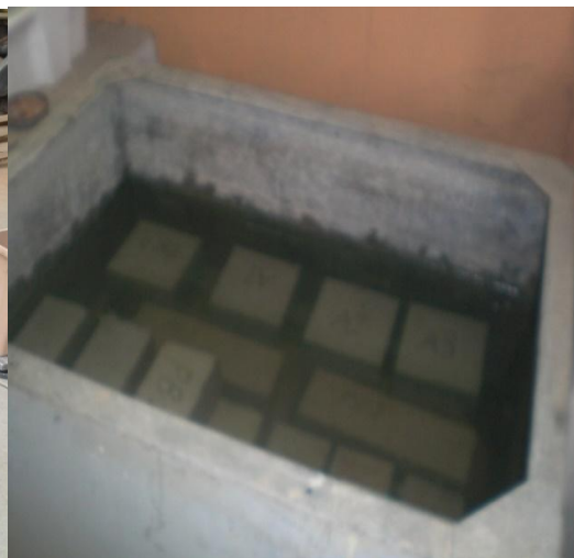
Fig. 2b. Curing of specimen in curing tank
