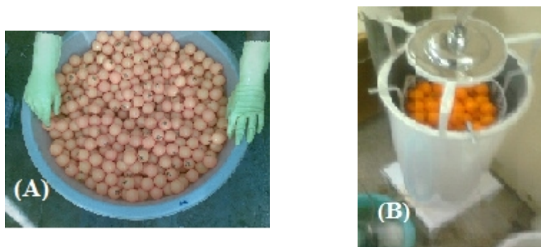
Fig. 1. (A) Plastic balls used as filter media (B) Trickling filter steel cage filled with plastic balls as a media
