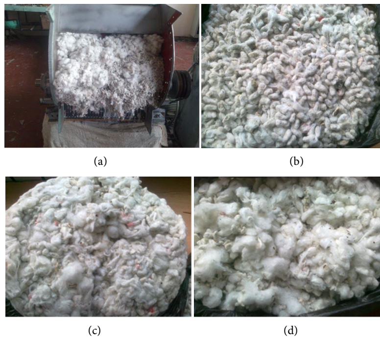
Figure 5. The composition of the seed roll in the roll box of the saw gin: (a) front view of the seed roll in the roll box, (b) bare seeds, (c) semi-ginned seeds, (d) non-ginned seeds.
