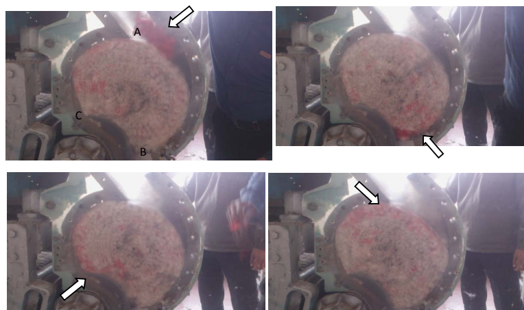
Figure 3. Designation of the roll box area on the side wall of the gin stand and the movement of the cotton.
